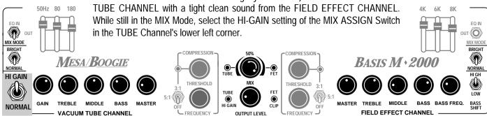
Set the controls in both channels to the setting shown in the above illustration. For this example, we have chosen a medium overdrive sound to audition. Select the MIX Mode (if you have not already done so.)
